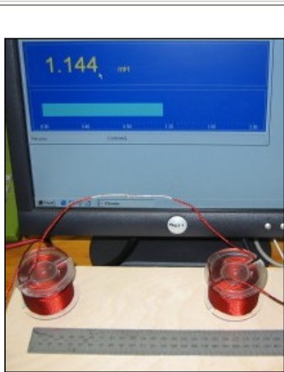
Fig. 1. Coils 20 cm apart: 1.144 mH
