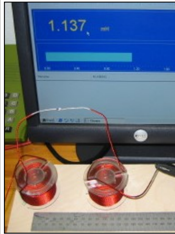
Fig. 2. Coils 10 cm apart: 1.137 mH.
