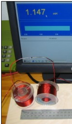
Fig. 5. Coils placed close as seen on picture: 1.147 mH.
