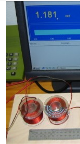
Fig. 4. Coils placed close as seen on picture, one coil turned upside down: 1.181 mH. Compare with fig. 3.
