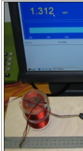
Fig. 7. Coils placed on top on one another, same orientation: 1.312 mH.
