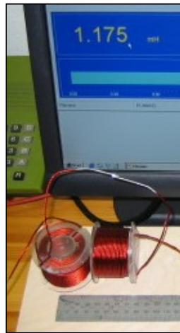
Fig. 6. Coils placed close as seen on picture: 1.175 mH
