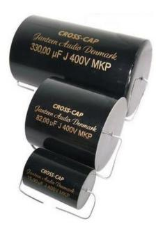
Technical specifications(according to manufacturer): "Single foil PP capacitor featuring extremely high quality German made foil, metalized with Aluminum and Zinc particles. Featuring terminal leads made from PCOCC copper (oxygen free). Voltage rating: 400VDC, Non inductive construction, Terminal leads are made from PCOCC copper (Pure Copper Ohno Continuous Cast Wire), Capacitance tolerance: +/- 5%, Loss factor: 1K 0.00002, Non-polarized capacitor".
